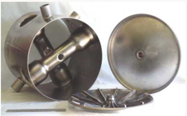
Figure 5A: Niobium elements of the 345 MHz double-spoke cavity prior to closure welds.
