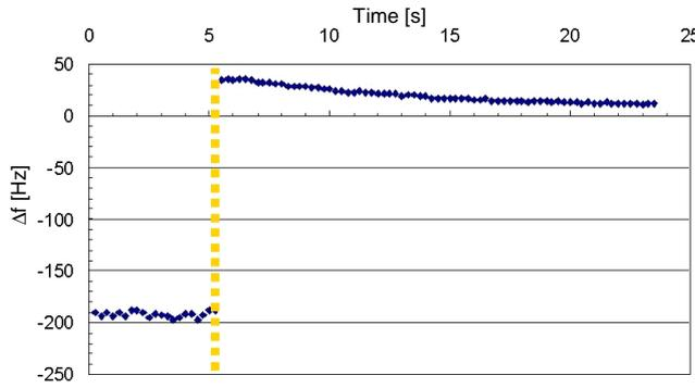
Figure 10: Typical frequency change induced in the SRFQ1 resonator by a heavy hammer stroke on the test cryostat outer vessel: however, no vibrations seem to have been induced (the resolution is 250 ms).
