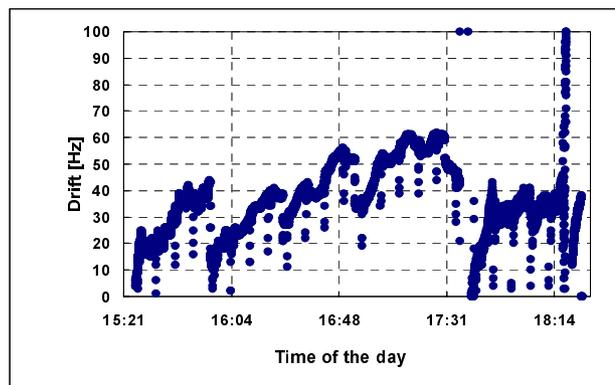
Figure 4: Natural excursions of unlocked SRFQ2 resonator frequency in a few hours time span; fast drifts are linked to the behaviour of the dryers of the lab cryogenic plant (around  $\pm 30 \text{ Hz/s}$ ), seen by the cavity through the gaseous He recovery line
