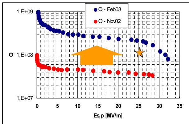
Figure 3: The Q curve recovered, after making the shape of the Nb sputtered end-plate to follow the shape of the Nb cavity (0.1 mm step induced by BCP)
