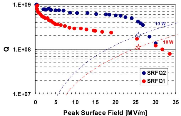
Figure 2: Q-curves of SRFQ1 and SRFQ2 exceed the design specifications (25.5 MV/m at 10 W)
