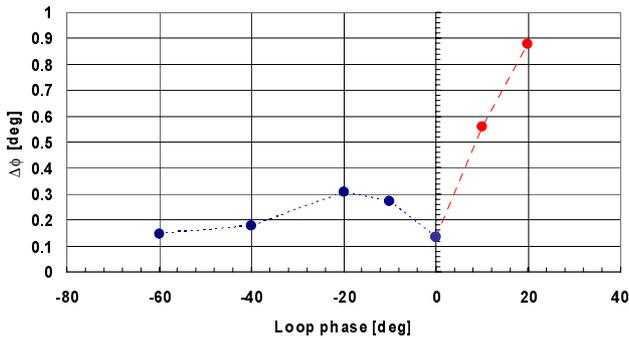
Figure 7: Average amplitude of the phase error of SRFQ1 versus the chosen value of the SEL loop phase of figure 6.
