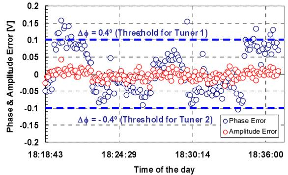
Figure 8: Typical excursions of phase and amplitude errors in the SRFQ's in the test cryostat: the phase error values, at which the mechanical slow tuners are moved, are shown.
