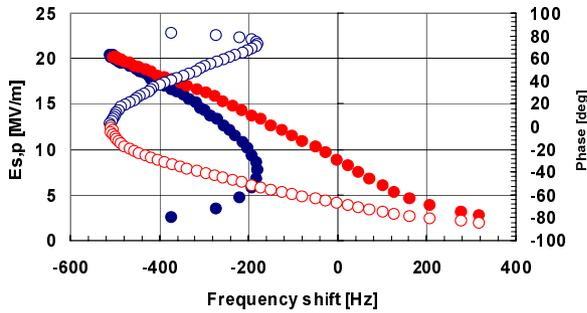
Figure 6: Folded resonance curves of the Lorenz detuned resonators: blue bullets correspond to the stable part of the curve, red bullets to the unstable one.
