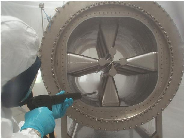
Figure 1: SRFQ1 during high pressure water rinsing, before being assembled into the final cryostat.
