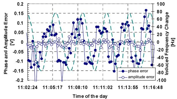
Figure 9: Sine function modulation of the master oscillator frequency, introduced to check the threshold velocity response of the mechanical tuners
