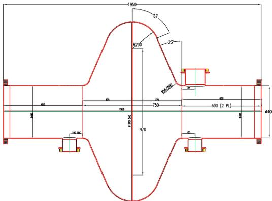
Figure 3: Dimensions of the 200 MHz Nb-Cu cavity.
