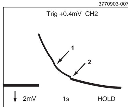
Figure 8: Two multipacting barriers are shown as two switches in the reflected power signal, indicated by arrows.
