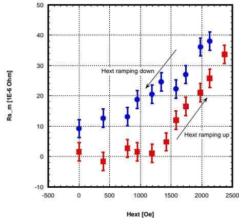
Figure 10: External magnetic field effect on the additional surface resistance of a 200 MHz Nb-Cu cavity.
