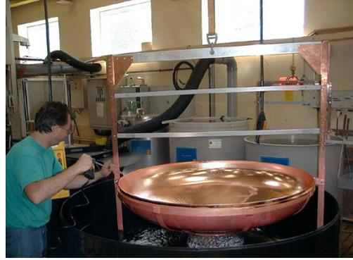
Figure 4: A half cell that is being rinsed.
