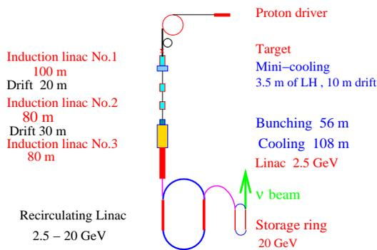
Figure 1: Schematic of the neutrino factory [2].
