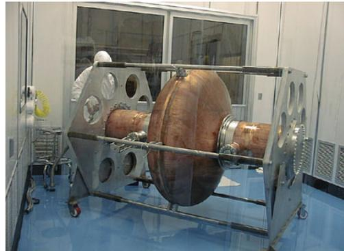
Figure 5: Assembling RF couplers on 200 MHz Nb-Cu cavity in the new LEPP clean room.
