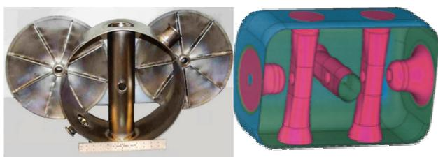
Figure 3: The spoke on the left is a simple design from ANL with a straight cylindrical spoke; the right resonator is a design from FZ Jülich with a rectangular cavity body.
