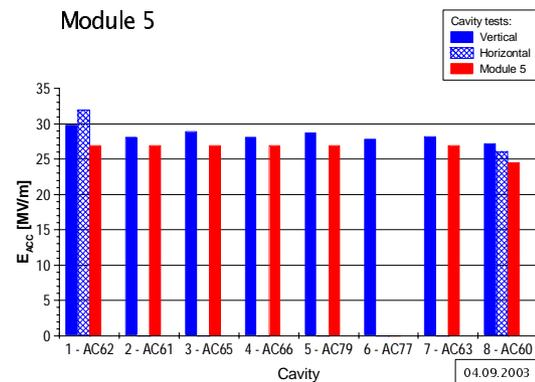
Figure 7: Cavity performance of module 5 at DESY
