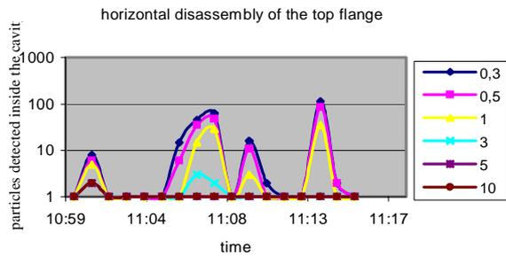
a) particles detected inside the cavity
