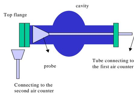
Figure 1: Sketch of particle measurement system
