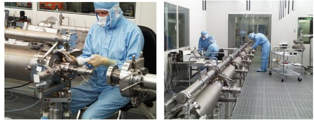
Figure 6: Cavity assembly in clean room
