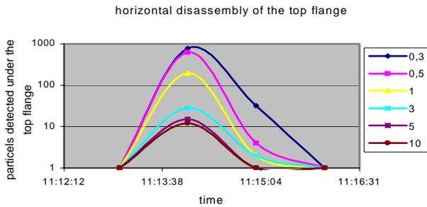
b) particles detected under the top flange (outside of the cavity) just after the top flange is removed
