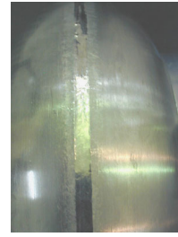
Fig. 4: Weld seam (4mm wide) at the equator
