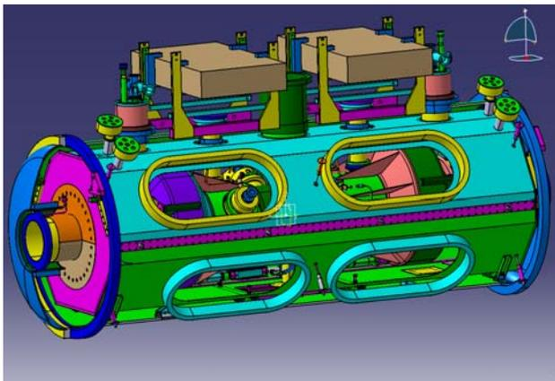
Figure 4 : Copper shield inserted in the cryomodule.
