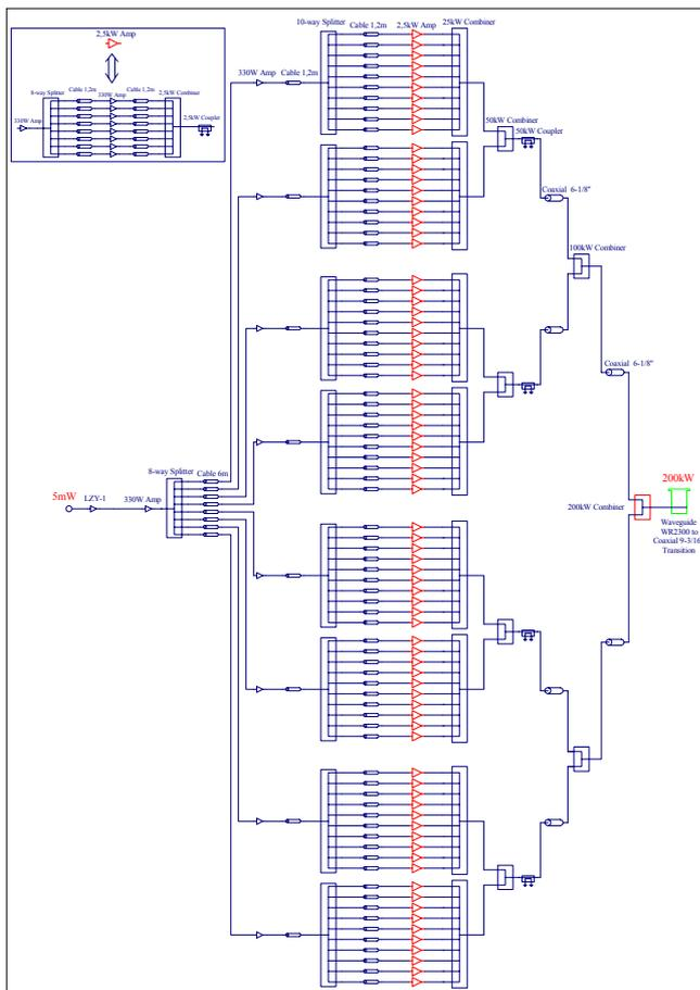
Figure 6: The RF power splitting and re-combination.
