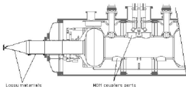
Figure 1 : SOLEIL cryomodule with HOM dampers.
