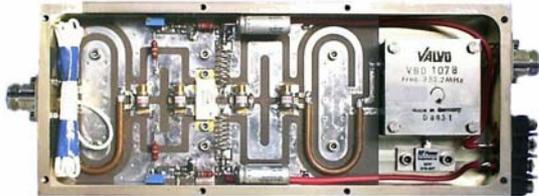
Figure 5: 315 W - 352 MHz amplifier module.
