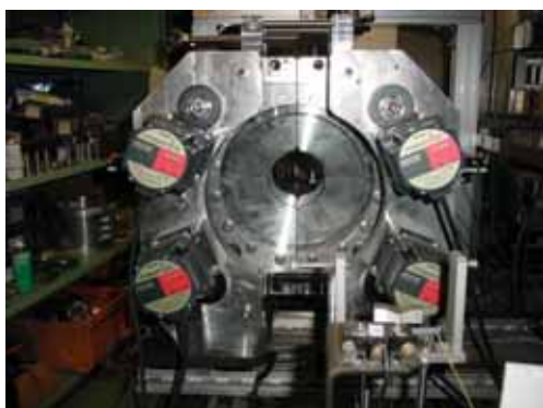
Figure 5: Clamping pads and stepping motors
