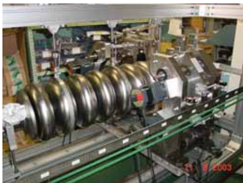
Figure 4: Pre-tuning equipment and a 9-cell Nb cavity
