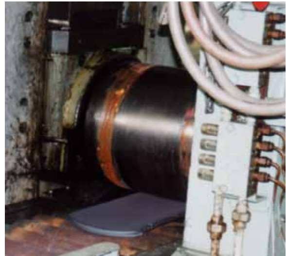
Figure 3: Hot rolling process of Cu/Nb/Cu clad sheet.
