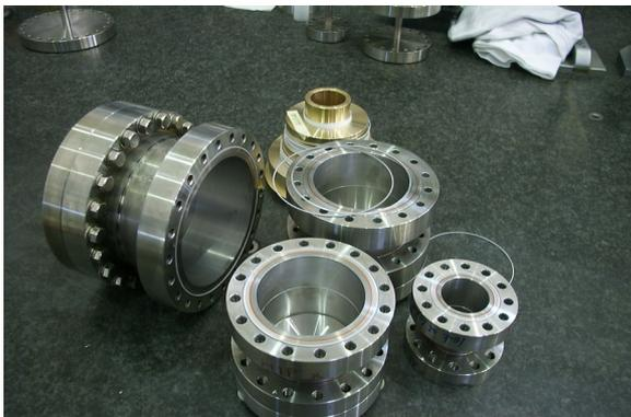
Figure 1: Pure aluminium fine ring sealing and stainless flanges bonded on niobium tubes.
