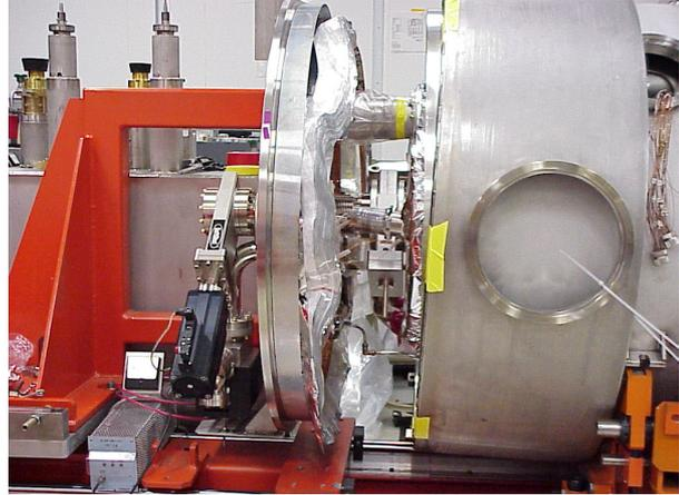
Figure 4: Enc Can Connection to the Cryomodule.
