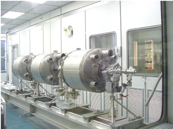
Figure 1: Medium Beta Cavity String in clean room.
