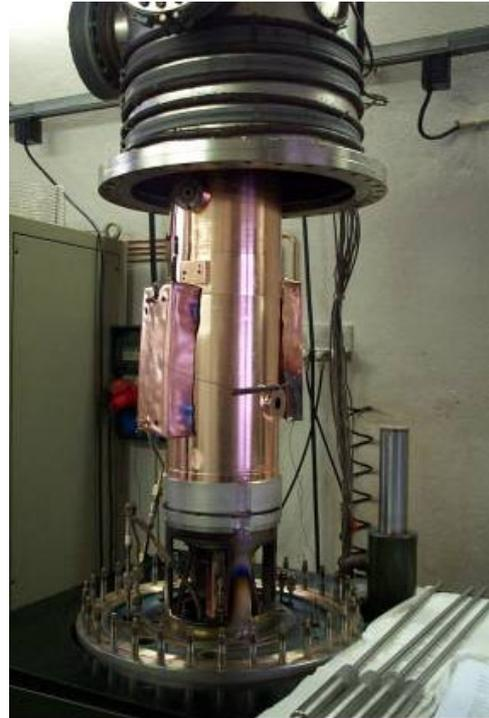
Figure 3: A medium  $\beta$  ALPI cavity mounted in the sputtering chamber.
