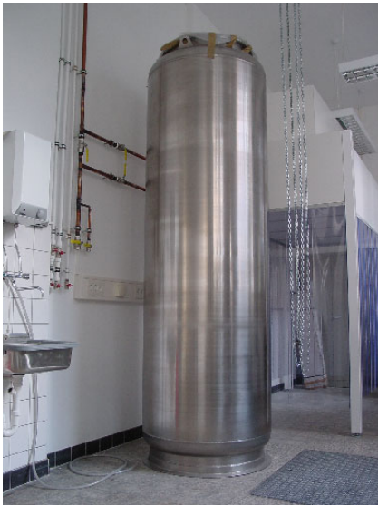
Figure 3: View into the new cryo laboratory in Frankfurt with a class 100 laminar flow box (background) and the 3 m vertical cryostat.
