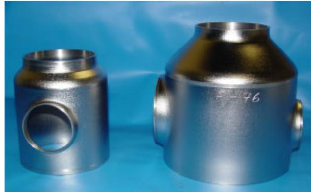
Figure 1: Raw end groups produced for SNS cavities by deep drawing and nipple pulling from one sheet.
