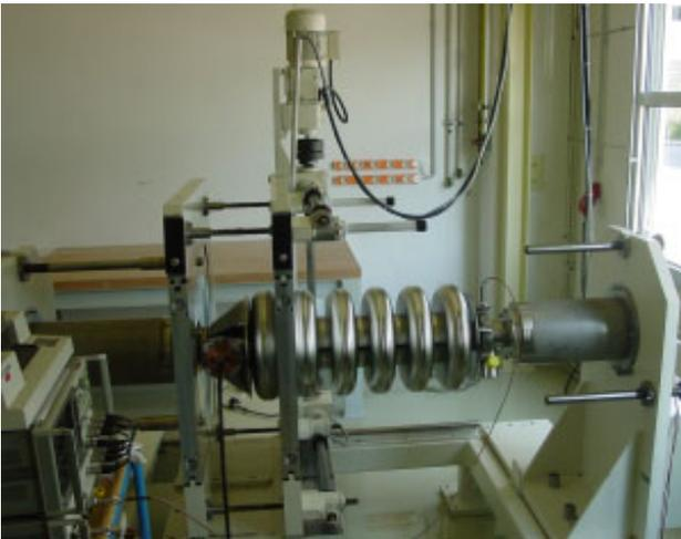
Figure 4: Tuning apparatus for SNS medium and high beta cavities. This machine now also allows tuning of TESLA cavities.
