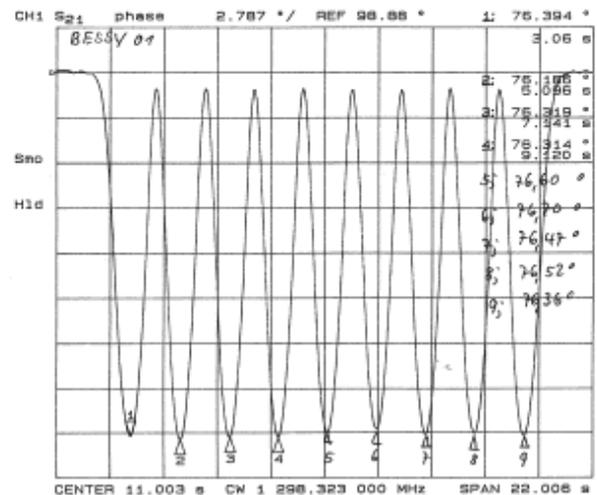
Figure 5: Field flatness of a TESLA cavity for BESSY after final welding (above) and after tuning (below).
