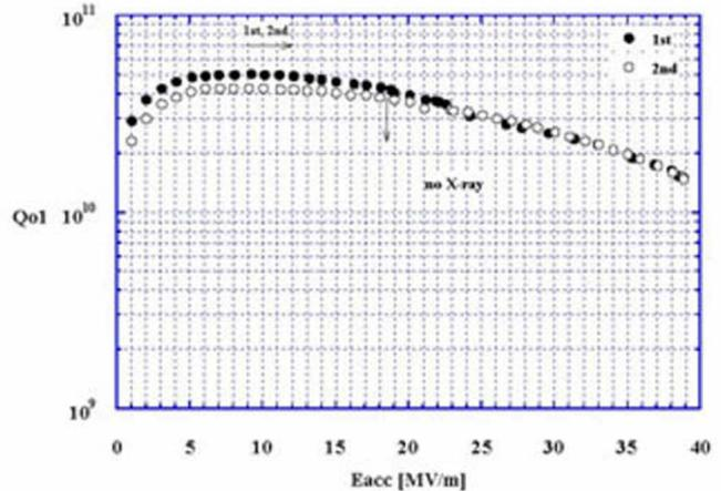
Figure 3: The cavity has been mechanically grinded for 100 microns, then barrel finished for 84 hours, vacuum annealed at 750 C for 3 hours, electropolished for 50 microns and then high pressure rinsed.
