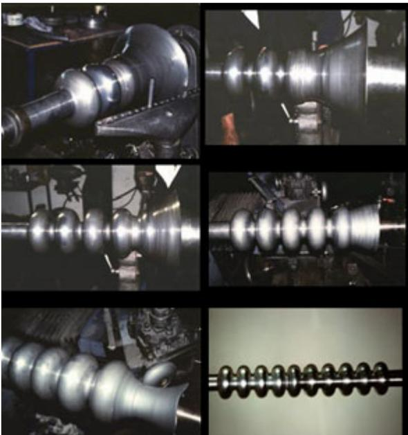
Figure 5: Spinning of a multicell cavity from disk.
