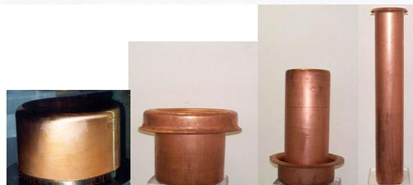
Figure 9: Reversal deep-drawing of seamless tubes.
