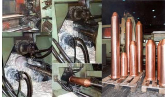
Figure 6: Flowturning of seamless Cu tubes.
