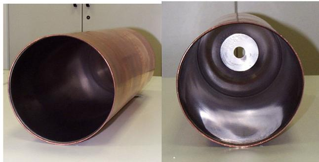
Figure 7: Niobium clad Copper seamless tubes.
