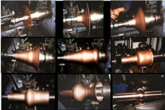
Figure 1: Spinning of a 1,5 GHz Copper cavity.
