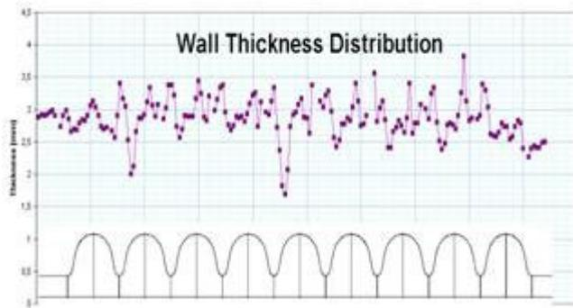
Figure 11: Wall thickness distribution for the nine-cell cavity.
