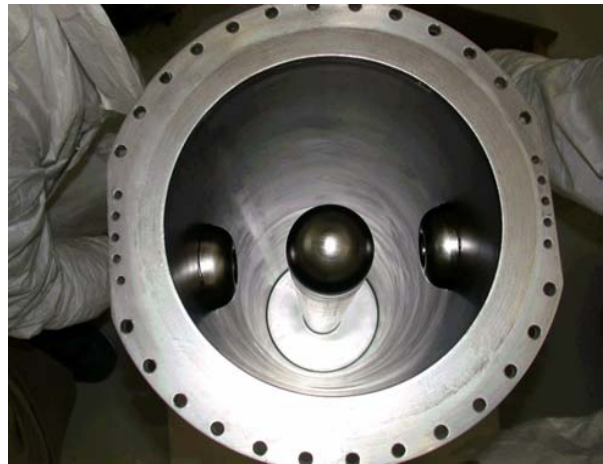
Figure 5: View of Niobium cavity with tuner plate
