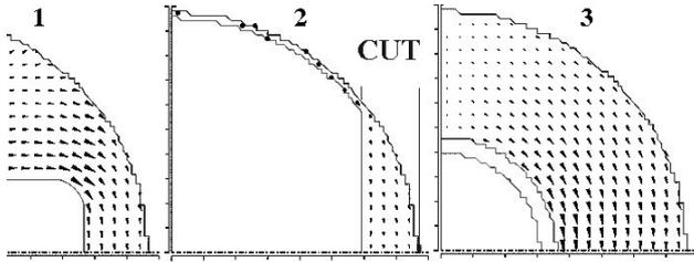
Figure 3: Magnetic fields for a CUT = 10 mm **1**, in the stub region 10 mm from the stem flange, **2**, through the stem flange and **3**, 5 mm from the stem flange and 115 mm from the shorting plate.
