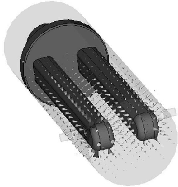
Figure 4: MWS simulation of the electric field distribution in DVOIKA with RAD = 16 mm.
