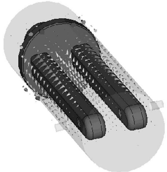
Figure 5: Magnetic field distribution in DVOIKA. MWS simulations for RAD = 16 mm.
