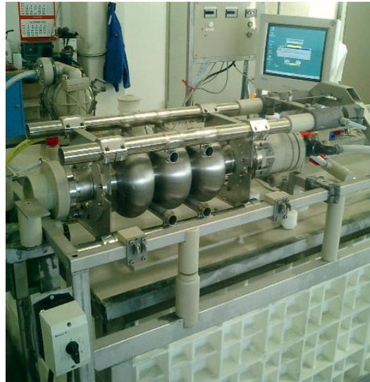
Figure 1: Setup for electropolishing
