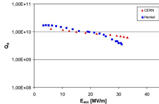
Figure 6: Behaviour of welded cavity after in-situ bake. The CERN test shows good performance of 33 MV/m. The first test after EP at Henkel was suffering from a vacuum leak. The cavity degradation starting at 20 MV/m is due to this problem. The maximum gradient is 31 MV/m. A new test is under preparation.
