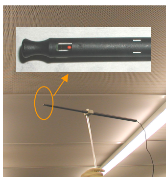
Picture 2: Detailed view on set up for air velocity measurements
