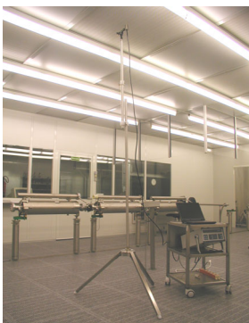
Picture 1: Set up for filter Leak test
