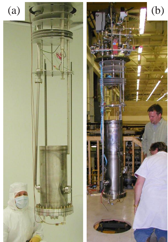
Figure 5: Photographs of (a) \beta_m = 0.16 QWR and (b) \beta_m = 0.085 QWR on the RF test stand.
