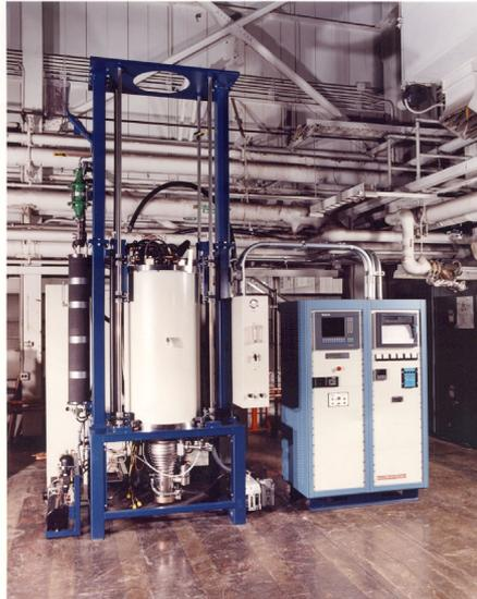
Figure 2: ANL hydrogen/vacuum furnace.
