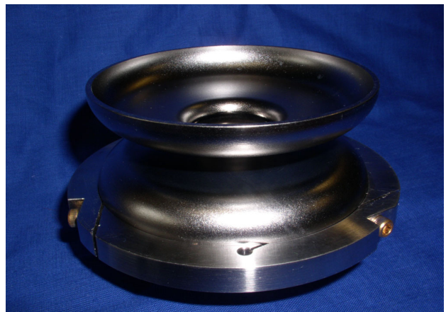
Figure 5 (b): Half-cells set up for internal weld pass
