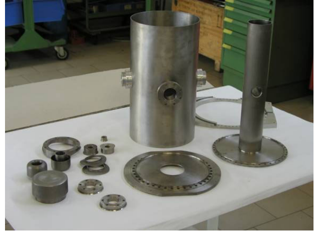
Figure 3: Resonator parts before welding.
