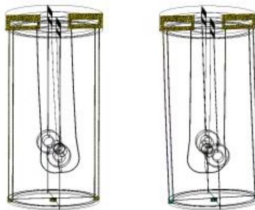
Figure 2: Lower frequency mechanical modes from I-DEAS
