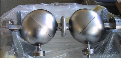
Figure 3: Niobium spherical cavities (variable coupling)
