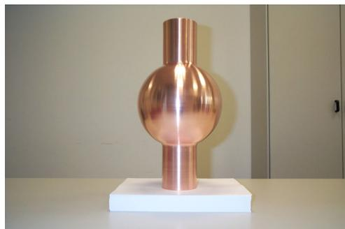
Figure 8: Single-cell, seamless, copper cavity
