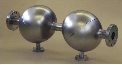
Figure 2: Niobium spherical cavities (fixed coupling)
