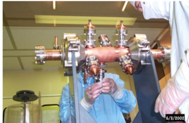
Figure 7: Super-3HC cavity assembling in clean room at Saclay
