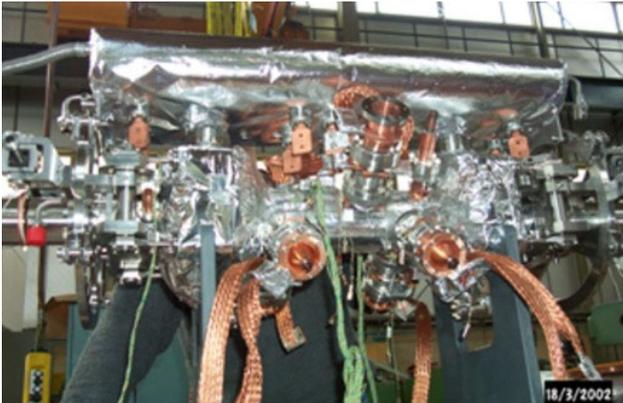
Figure 8: Cold mass assembling in the workshop.
