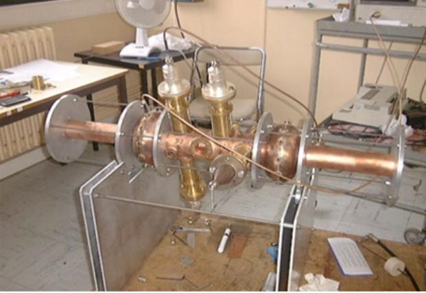
Figure 1: Model cavity for HOMs damping optimisation.
