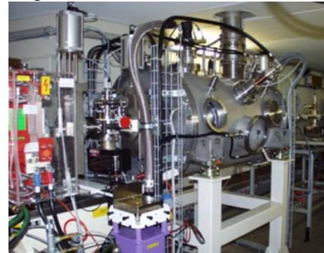
Figure 10: The cryomodule on SLS storage ring.
