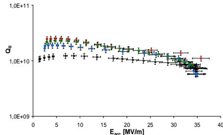
Figure 8: TESLA nine-cell cavities electropolished at KEK/Nomura Plating.
