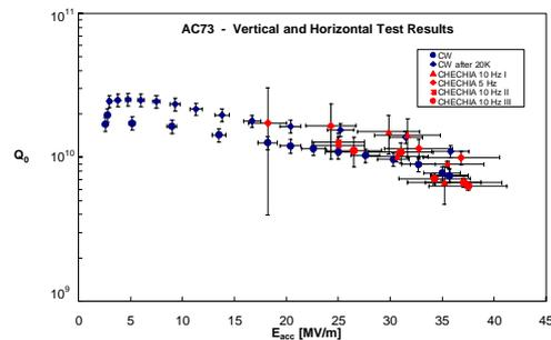
Figure 9: High power test of an electropolished TESLA nine-cells.
