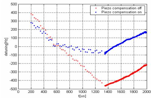
Figure 10: Compensation of Lorentz-forces using piezoelectric tuners.
