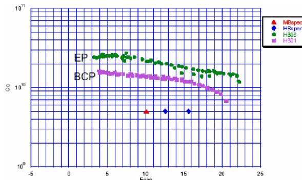
Figure 2: The electropolished SNS high beta cavity improved its performance as compared to the test after etching [14].
