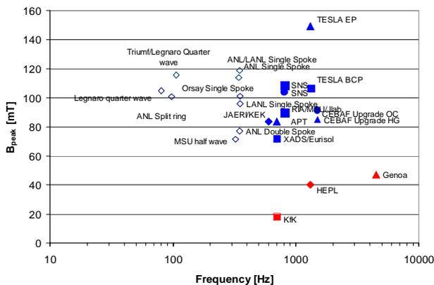
Figure 12: Maximum  $B_{peak}$  with compared between drift tube and elliptical cavities. Open symbols: Drift tube cavities, closed symbols: elliptical cavities. (Drift tube data is courtesy of Mike Kelly (ANL).)
