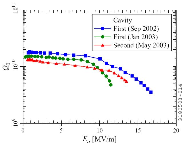
Figure 5: Results for RIA 805 MHz,  $\beta=0.47$ , six-cell cavities [17].
