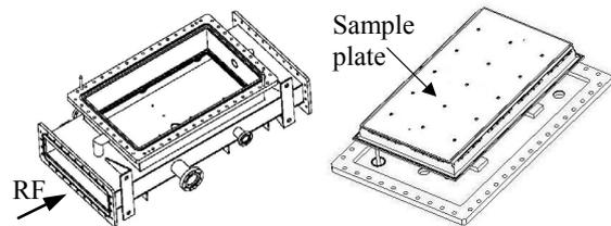
Figure 1: Schematic of the waveguide and of the sample plate mounted on the flange.
