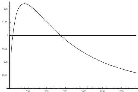
Figure 2: Secondary electron yield curve used for the simulations.
