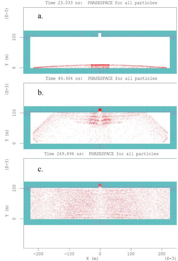
Figure 3: Evolution of a simulation with a single groove. a) Seeding the waveguide with electrons; b) First secondary electrons are created; c) After a long simulation time, the electrons are spread out independently of the starting conditions.
