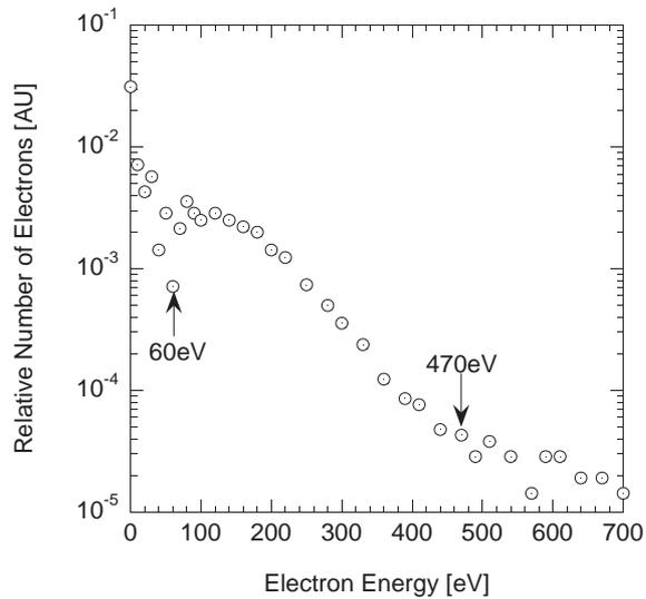
Figure 5: Electron energy spectrum for a forward power of 250 kW.
