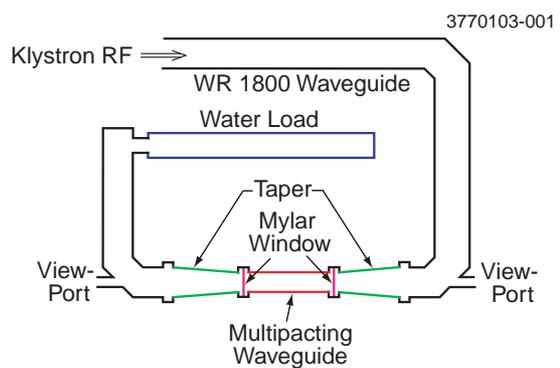
Figure 1: Layout of the rectangular waveguide multipacting experiment.
