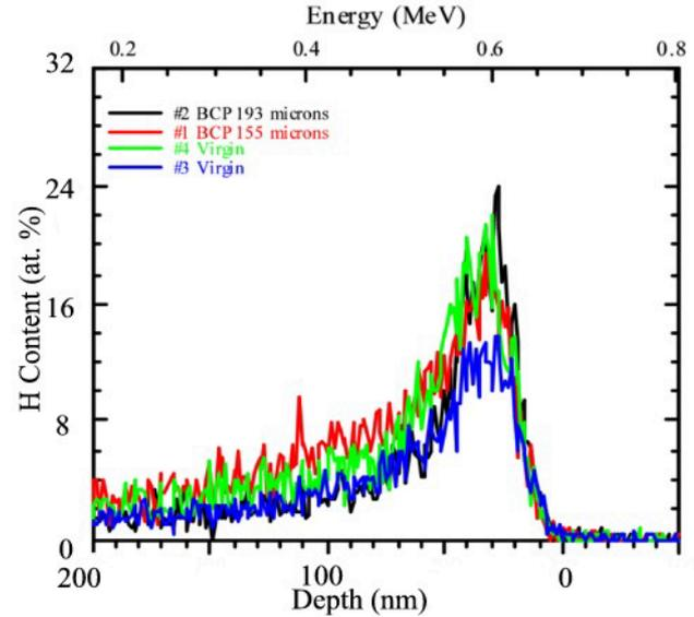
Figure 4: Depth profile of hydrogen for the non-treated (virgin) samples and those after BCP of 155 and 193 microns.
