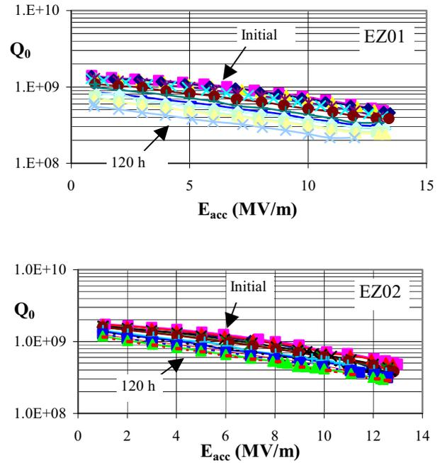
Figure 1: A collection of  $Q_0$ - $E_{acc}$  curves of our 350-MHz spoke cavities EZ01 (top) and EZ02 (bottom) measured at 4 K after every 12 hours of holding the cavity at 100 K up to 120 hours.
