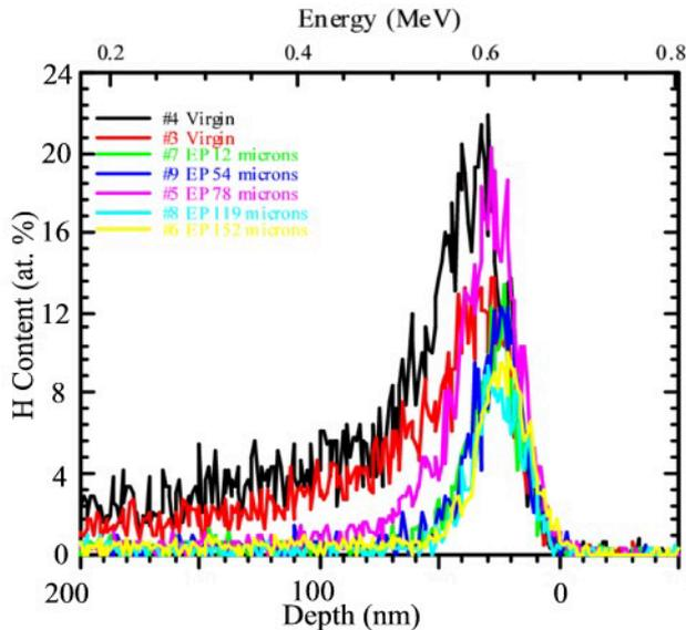
Figure 6: Depth profile of the hydrogen for electropolished (EP) samples as compared to the virgin samples.
