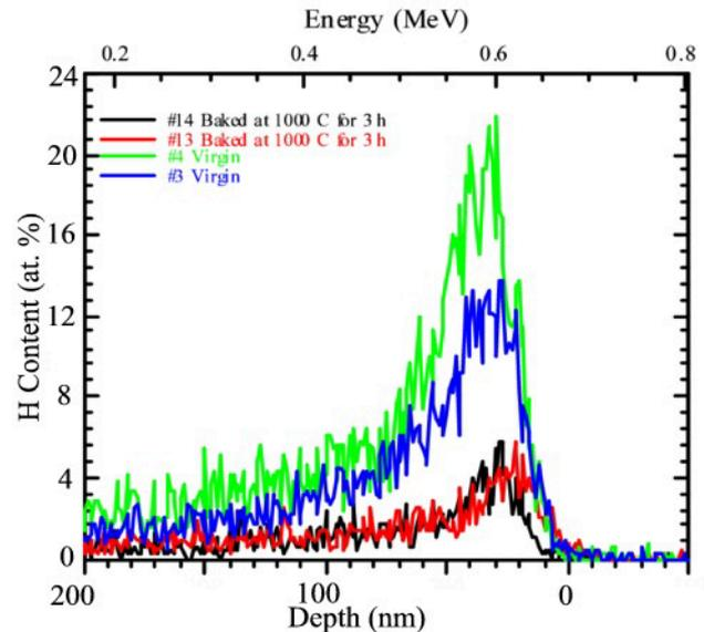
Figure 5: Depth profile of the hydrogen for the non-treated (virgin) samples and those baked at 1000 °C for 3 hours.
