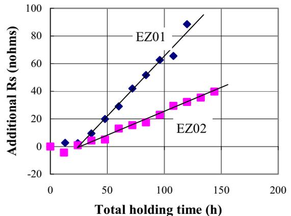
Figure 2: Additional surface resistance due to Q disease as a function of accumulated holding time at 100 K. The data was taken at  $E_{acc}=4$  MV/m.
