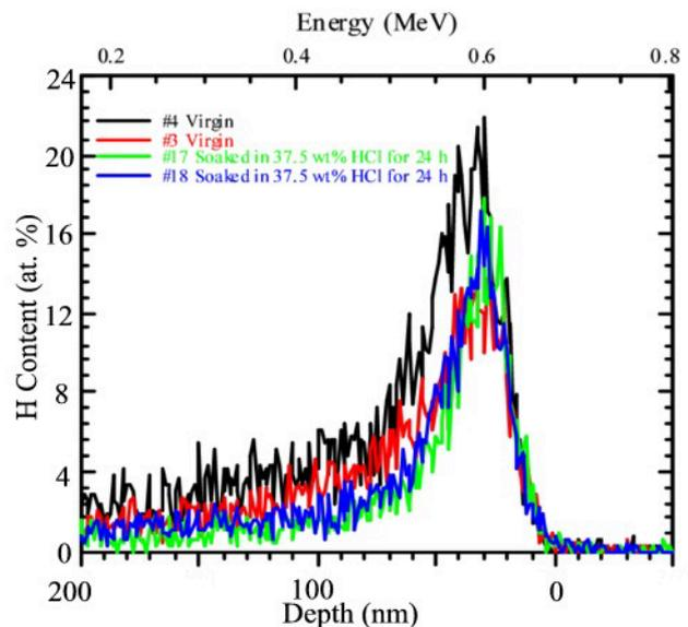
Figure 8: Depth profile of the hydrogen for the samples soaked in 37.5 wt% HCl for 24 hours as compared to the virgin samples.
