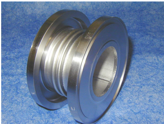
Figure 7: Bellows with welded on Nb55Ti flanges.
