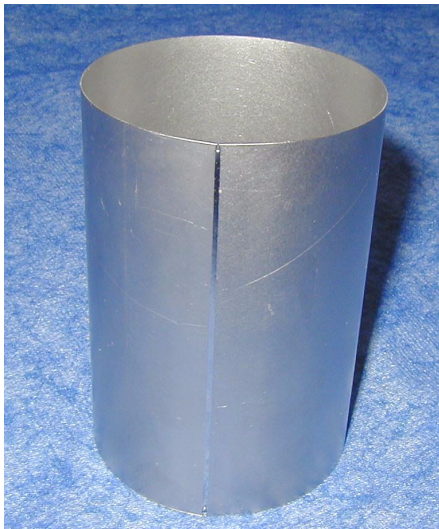
Figure 3: Welded thin wall niobium tube.
