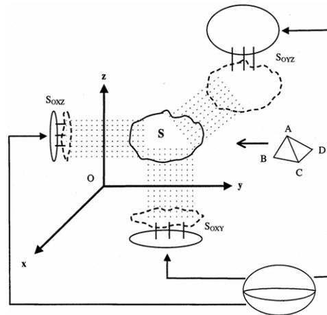
Figure 1: Analyzed surface projection and its ellipsoid projection on the three planes. In this analysis the analyzed surface is considered as composed of elementary micro-facets ( $ABCD$ ) from [3].
