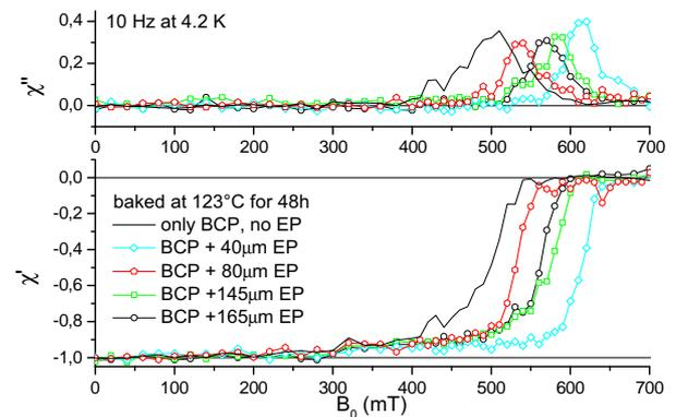
Figure 7: The ac susceptibility of electropolished samples after baking at  $123^\circ\text{C}$  for 48 hours.
