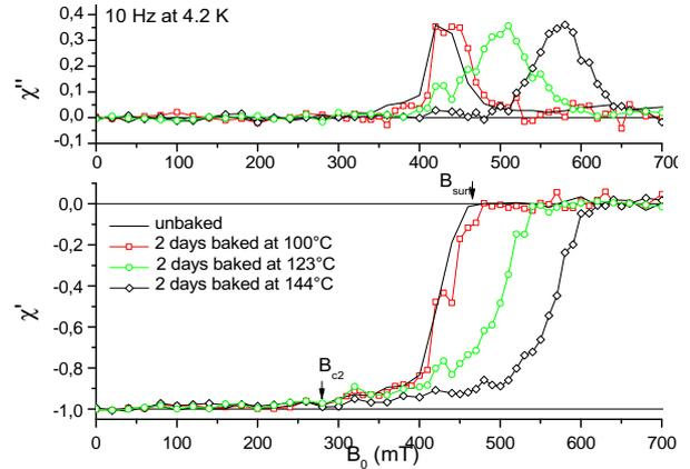
Figure 2: Imaginary ( $\chi''$ ) and real part ( $\chi'$ ) of the ac susceptibility of an unbaked sample and three samples baked for 48h at different temperatures. The values  $B_{c2}$  of the bulk material and  $B_{\text{surf}}$  are indicated for the unbaked sample.
