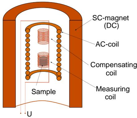
Figure 1: Schematic drawing of the experimental setup.
