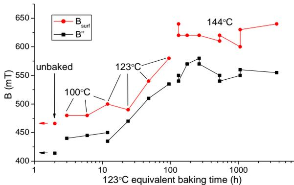
Figure 4: The surface critical field  $B_{\text{surf}}$  and the field  $B''$  where  $\chi''$  assumes its maximum, plotted against the equivalent baking time at the reference temperature of  $123^\circ\text{C}$ .
