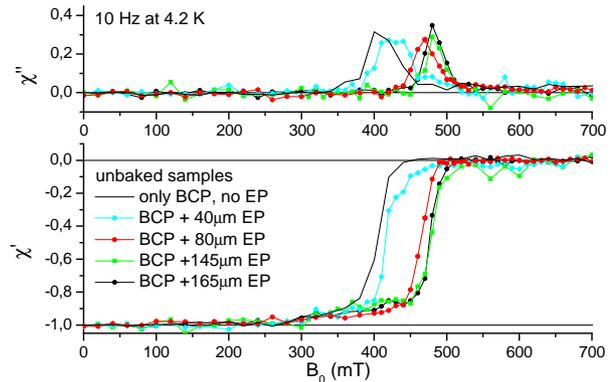
Figure 6: The real and imaginary parts of the ac susceptibility of electropolished samples in comparison with an unbaked BCP-sample.
