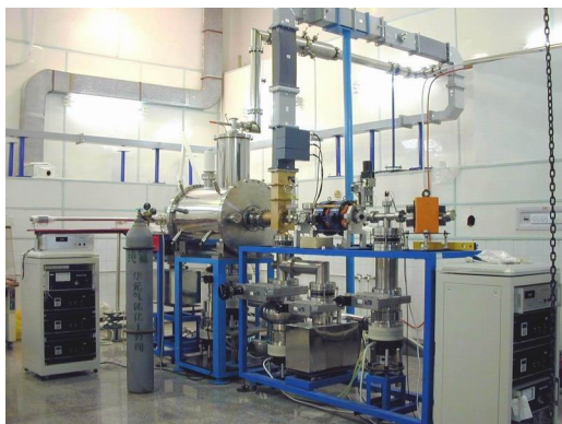
Figure 2: DC-SC photoinjector test facility.
