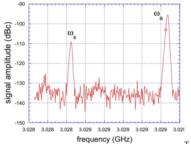
Figure 5: Rejection of the Symmetric mode operated by the control loop
