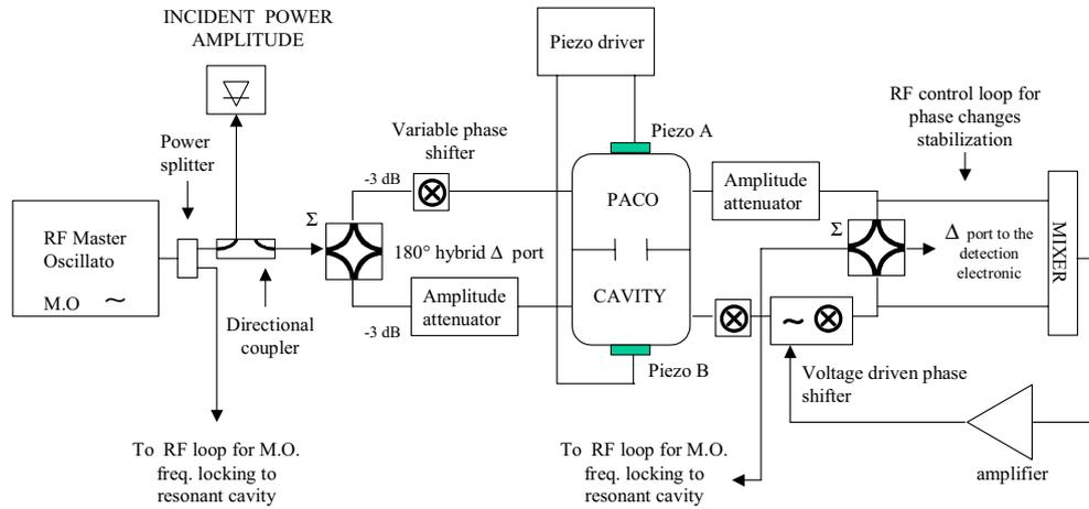
Figure 2: Schematic view of the RF circuit.
