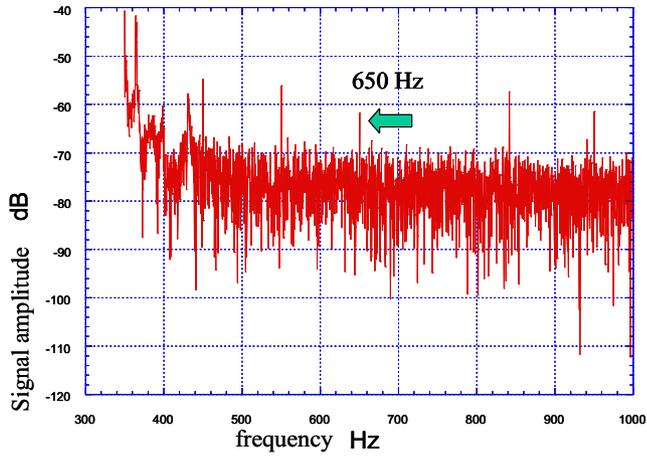
Figure 8: Mechanic resonant modes from 350 Hz to 1 kHz
