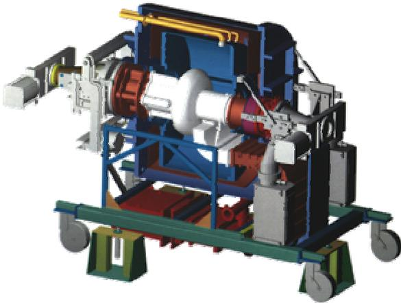
Figure 2: Cutaway view of superconducting module.
