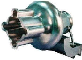
Figure 1: 500 MHz Cornell cavity.
