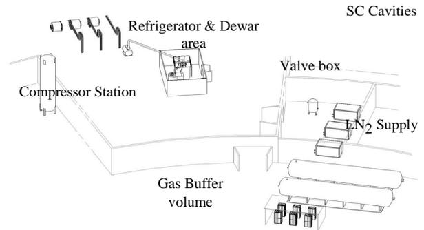
Figure 3: Schematic showing the Cryogenics layout.
