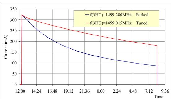
Fig. 3: Beam current decay with SUPER-3HC active (red) and parked (blue).
