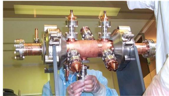
Fig. 1: SUPER-3HC cavity during assembling at CEA.
