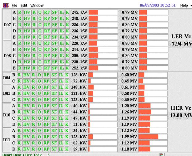
Figure 2: RF klystrons of KEKB. Eight klystrons of D10 and D11 sites provide the RF power to the SC cavities.
