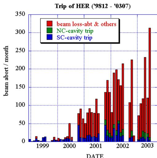
Figure 4: Total trips of KEKB-HER. The number of trips is increasing as the beam intensity improved, however, trips due to RF have never been affected by the intensity.
