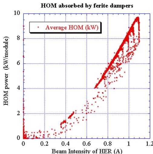
Figure 3: The total HOM power absorbed by a pair of ferrite dampers of one SC module.
