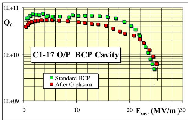
Figure 2:  $Q_0$  ( $E_{acc}$ ) before and after  $O^+$  plasma treatment.
