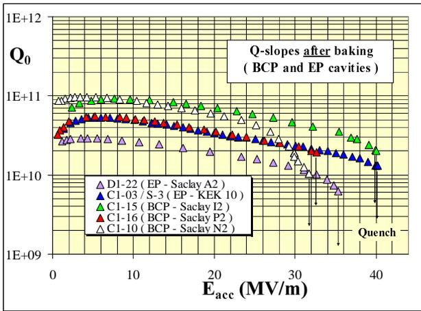
Figure 6:  $Q_0$ -slope Improvement after baking.
