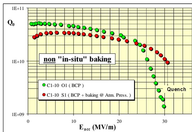
Figure 1: Q<sub>0</sub>-slope Improvement for BCP cavity by using a non “in-situ” baking.
