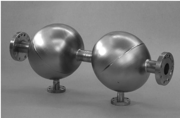
Figure 3: PACO, the 633 mm long superconducting resonator for the detection of gravitational waves.
