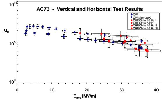
Figure 3: Excitation curves of the electro-polished high-performance 9-cell TESLA cavity AC73 in vertical (cw) as well as horizontal (CHECHIA) tests. The systematic rms errors in the determination of the accelerating field and the quality factor are indicated.
