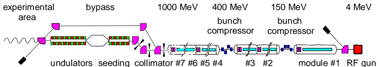
Figure 5: Schematic layout of the superconducting TTF linac for phase II. The electron beam direction in this picture is from right to left.
