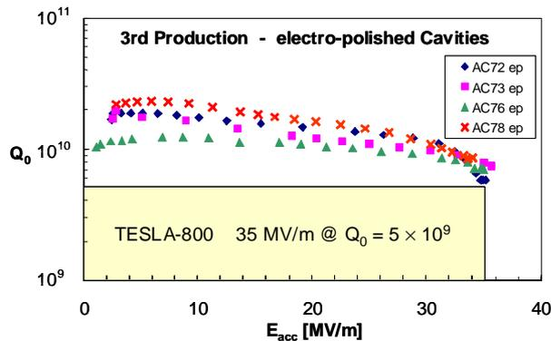
Figure 2: Excitation curve of high-performance 9-cell TESLA cavities treated with EP. The cavities are cooled by superfluid helium at 2 K.
